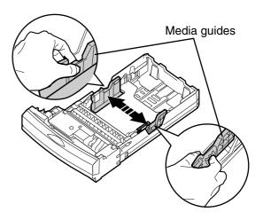
3 Slide the length guide unit to adjust it to the media length. Slide the length guide unit (2) while pressing the PUSH mark (1) to extend it.
